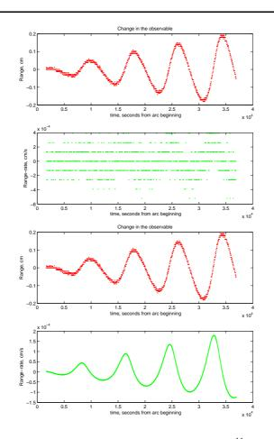
**Fig. 6** Range and range rate differences due to a change by  $10^{-11}$  of the  $C_{22}$  harmonic coefficient. Top: the range rate computed as range difference divided by the integration time of 30 s, eq. (8), is obscured by the rounding off. Bottom: the range rate computed as an integral, eq. (9), is smooth; the difference is marginally significant with respect to the measurement accuracy.
