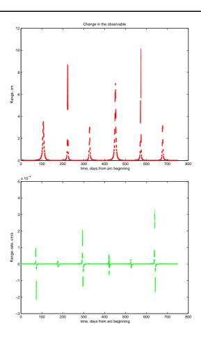
Fig. 4 Differences in range (top) and range rate (bottom) by using an order 1 and an order 2 post-Newtonian formulation ( $\gamma = 1$ ); the correction is relevant for BepiColombo, at least when a superior conjunction results in a small impact parameter b. E.g., in this figure we have plotted data assumed to be available down to  $b \simeq 3R_0$ . For larger values of b the effect decreases as  $1/b^2$ .
